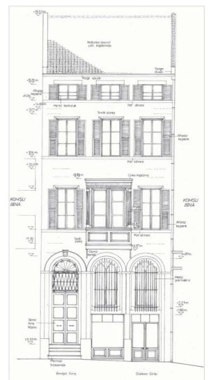
Fig. 7 The reconstruction drawing of the facade of Arapoğlu Mansion, Drawing by B. S. Yalçın, 2003
